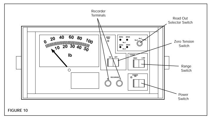
NOTE: Start the machine in operation with a web in place. Set the TM140A Power Switch to ON.
